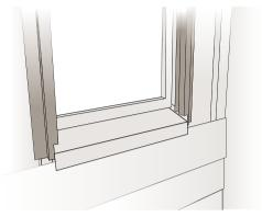
Fix external window (asymmetric) profiles to the sides of the window.
