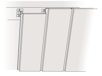
Screw Click Clips onto every batten to fix the edge of the plank into place.
