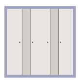
Fix end profiles horizontally at the top and bottom of each run of planks. Drill weep holes to allow for drainage.
