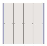
Fix vertical connection profiles, click external corner profiles or lap external corner profiles.
