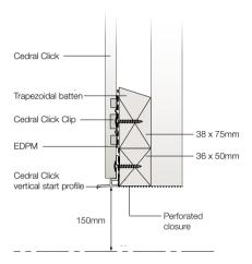
Rest the bottom of the planks on the vertical start profile. Please note the bottom batten must be trimmed to allow this to fit correctly as per the diagram above. This must also be repeated between joints.
