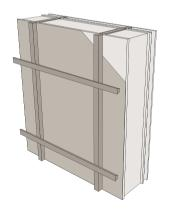
Horizontal counter battens should then be fixed.
