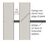
Place front planks over the rear plank ensuring the overlap is a minimum of 60mm.
