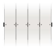
Planks are laid next to each other, with a 3-12mm open gap between each.
