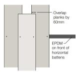
Screw through the face of the front planks penetrating both planks and screwing into the timber. Fixings must be 20mm minimum from the edge of the plank and again all planks must be fixed twice to every batten.
