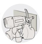
Trial nailing should be conducted to set the depth of the fixing. Respect the minimum 20mm edge distance.
