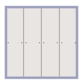
Fix end profiles to the top and bottom of each section of planks. Drill weep holes to allow for drainage.
