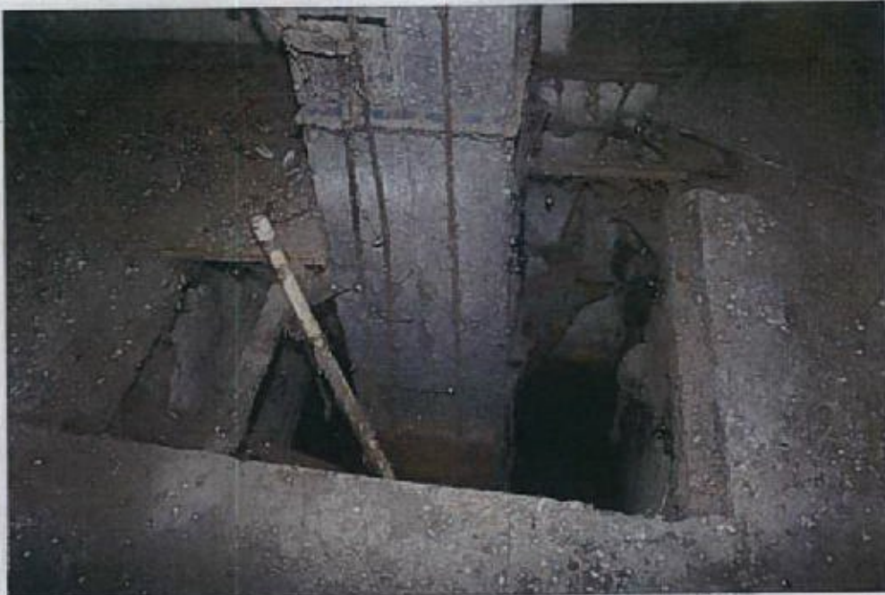
The base of the bucket elevator. Product was poured into the pit to be lifted up.
