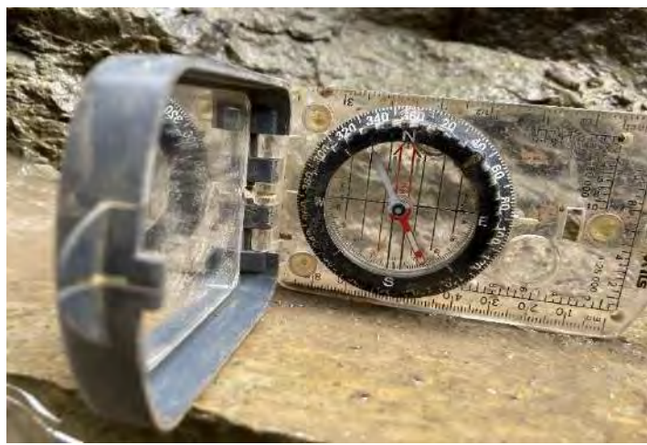
Plate 36 | TPA. The dip of the bedding planes measures at c.18° down to the E.
