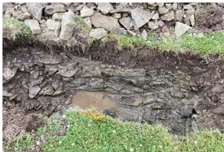
Plate 35 | TPA, post-soakaway testing, structure of the rock more visible with some tight fractures.
