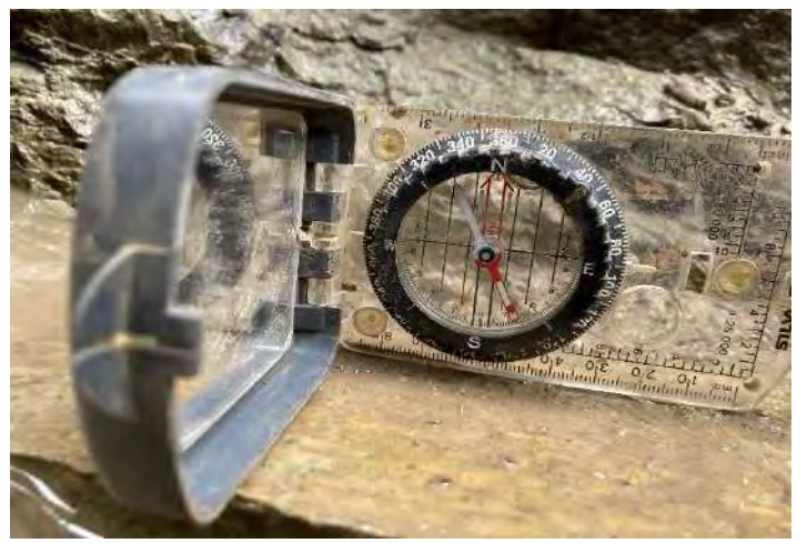
Plate 35 TPA, post-soakaway testing, structure of the rock more visible with some tight fractures. Plate 36 TPA. The dip of the bedding planes measures at c.18° down to the E.
