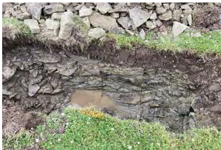
Plate 35 TPA, post-soakaway testing, structure of the rock more visible with some tight fractures. Plate 36 TPA. The dip of the bedding planes measures at c.18° down to the E.
