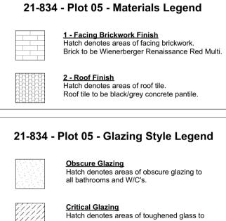
all window glazing below 800mm from the internal floor finish level, and to all doors and sidelights glazing below 1500mm from the internal floor finish level
