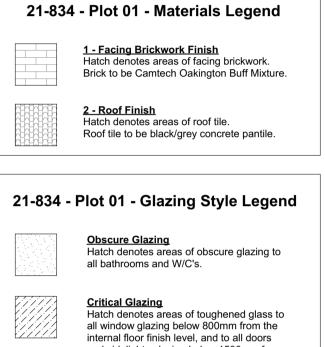
and sidelights glazing below 1500mm from the internal floor finish level
