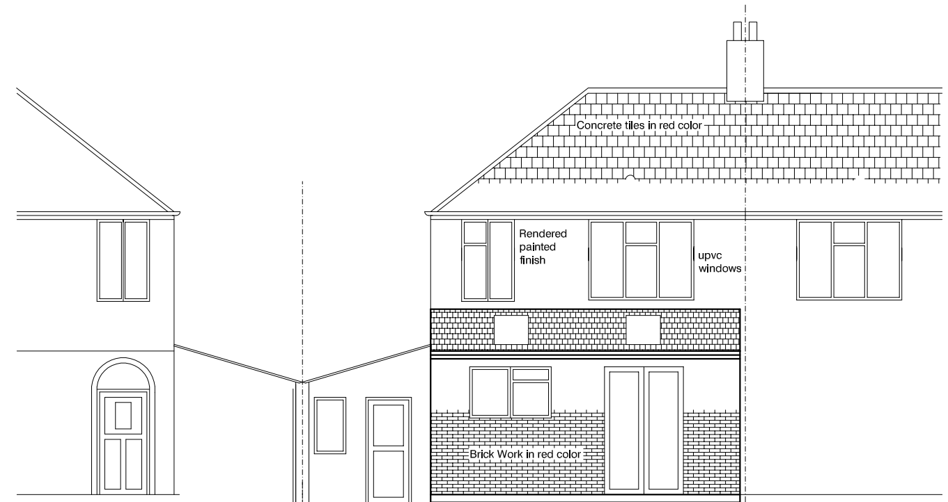
EXISTING REAR ELEVATION
