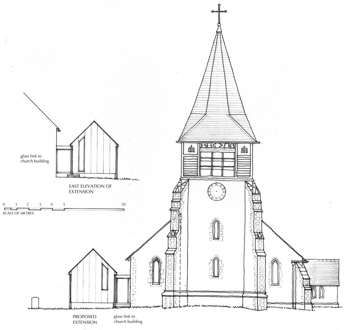
PROPOSED EXTENSION walls and roof zinc clad to harmonise with stone and flint of the church. Metal framed windows painted dark grey.
