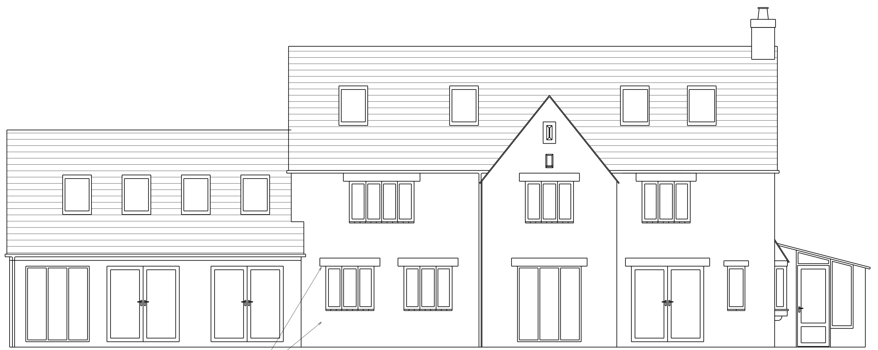
EXISTING REAR ELEVATION, SOUTH FACING
