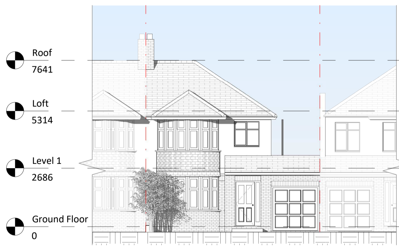
5 Existing Front Elevation 1 : 100
