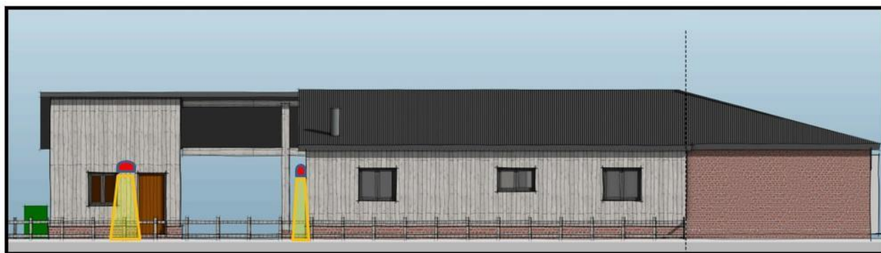
Elevation drawing with new lamps and predicted light spillage (view to east)
