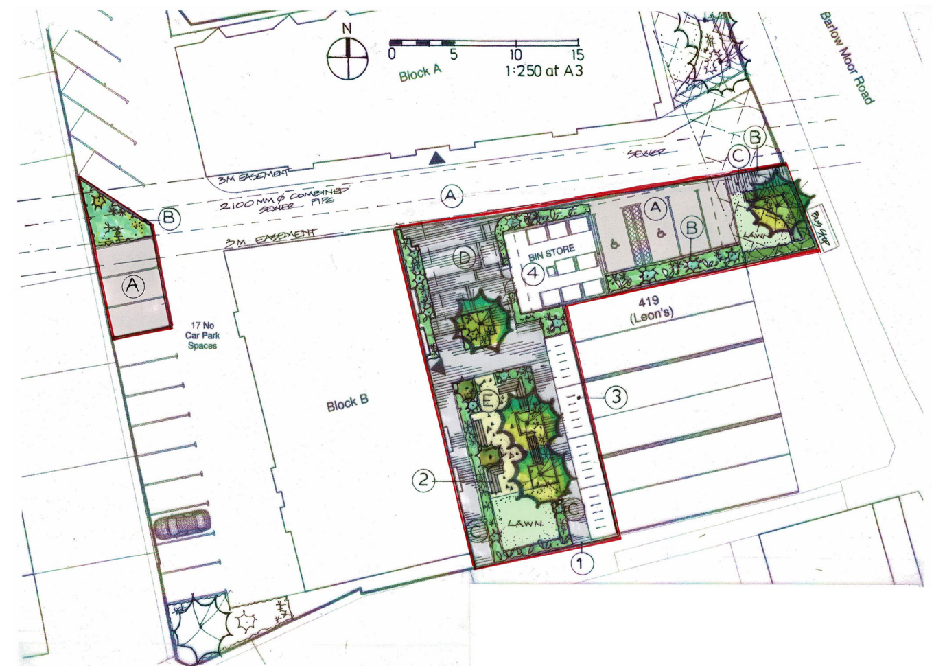
Excerpt of Margaret Twigg Landscape Architect's drawing, '479.03 Landscape Proposals to New Bin Store, Cycle Stores & Courtyard'.
