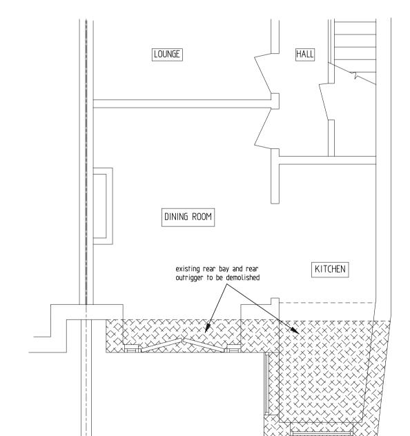
Existing Ground Floor Plan Scale 1:50
