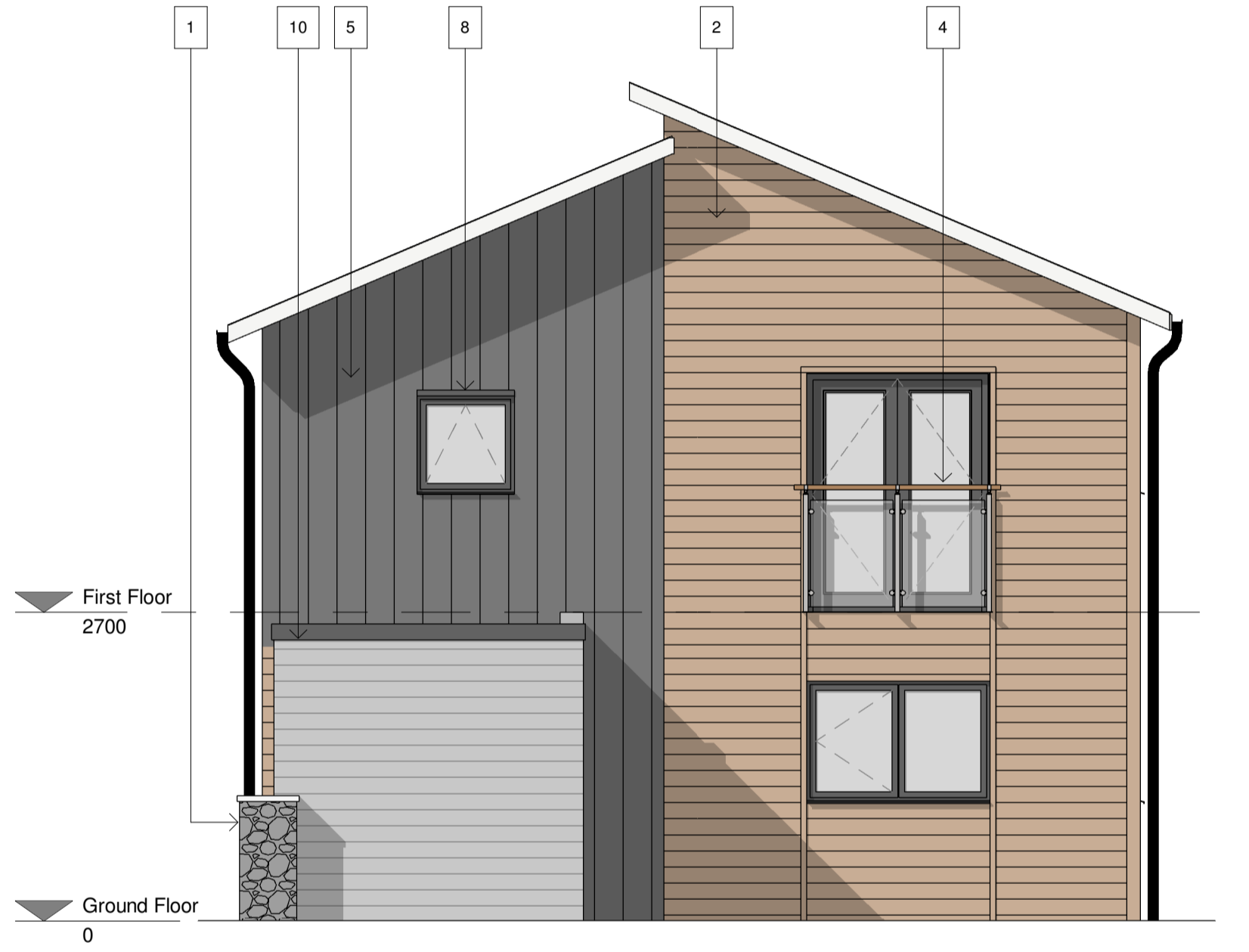
Principal Elevation - Front facing elevation (including external terraces, front entrance) 1:50 Scale
