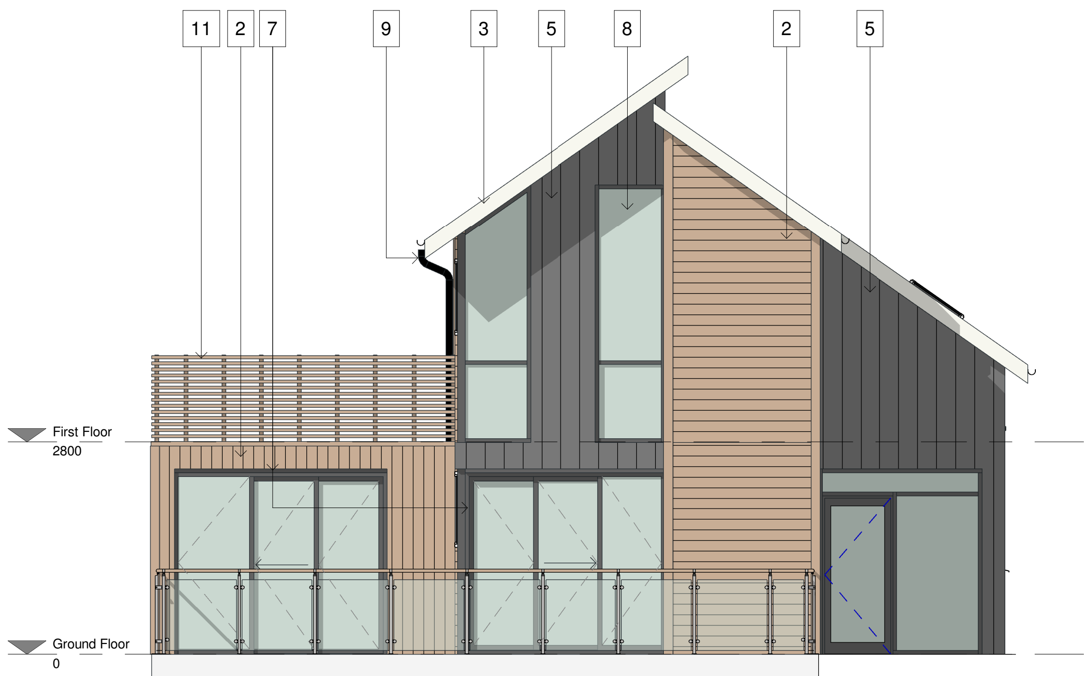
Principal Elevation - Front elevation (including external terraces, glazed screens to master bedroom/lounge) 1: 50 Scale
