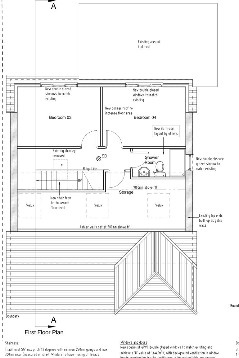
making a uniform angle on plan and going to be nowhere less than 50mm. Min 2000mm headroom throughout. Balustrading to staircase to be 900mm high vertically above pitch line with spindles spaces at max 100mm distance apart. Width 275mm.
