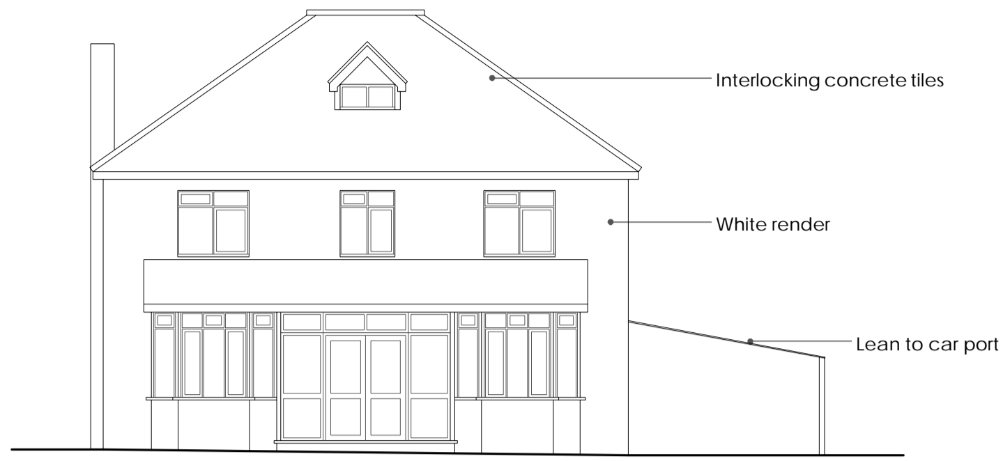
Front Elevation As Existing
