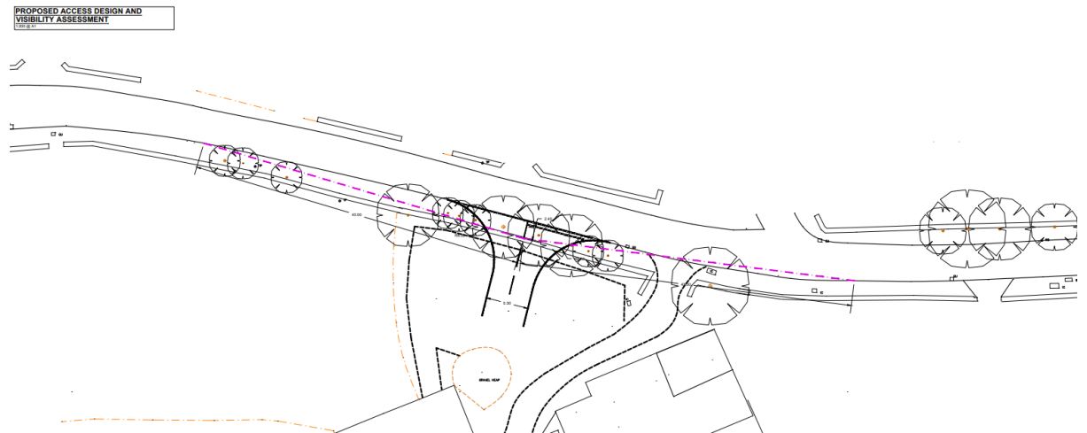
Figure 4. Extract of plan showing the extent of the visibility splay on Comb Hill Road.
