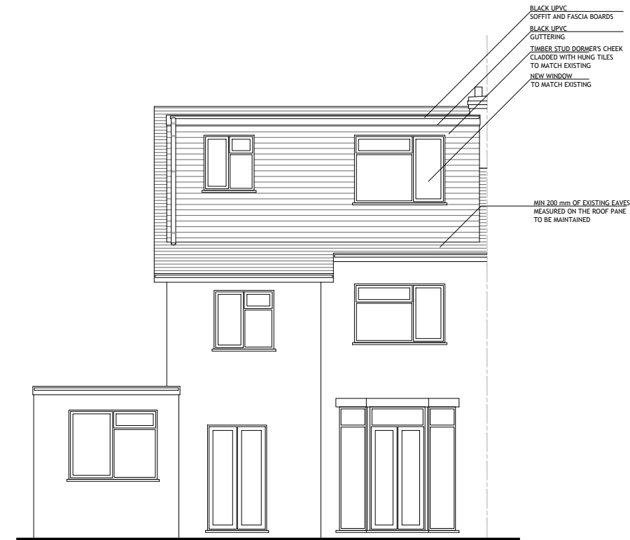
PROPOSED REAR ELEVATION SCALE 1:50
