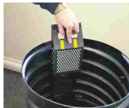
Slide the front plate with Smart Pak in down onto the back plate
