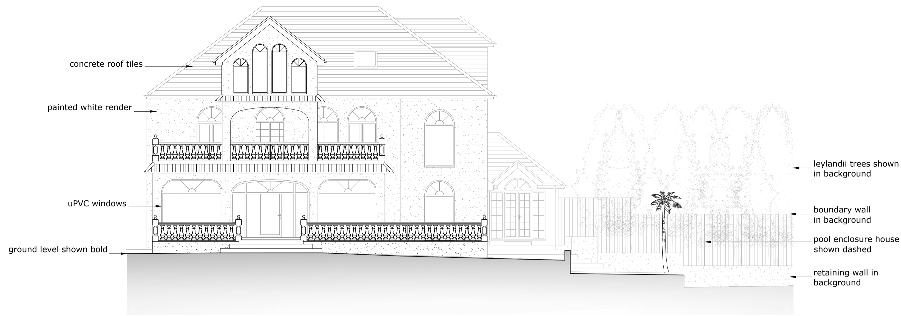
existing south elevation 1:100
