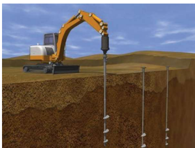
Typical helical mini-pile installation method
