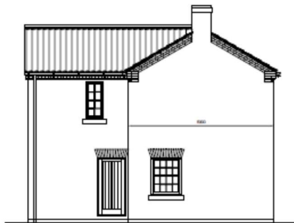
Proposed side elevation facing west
