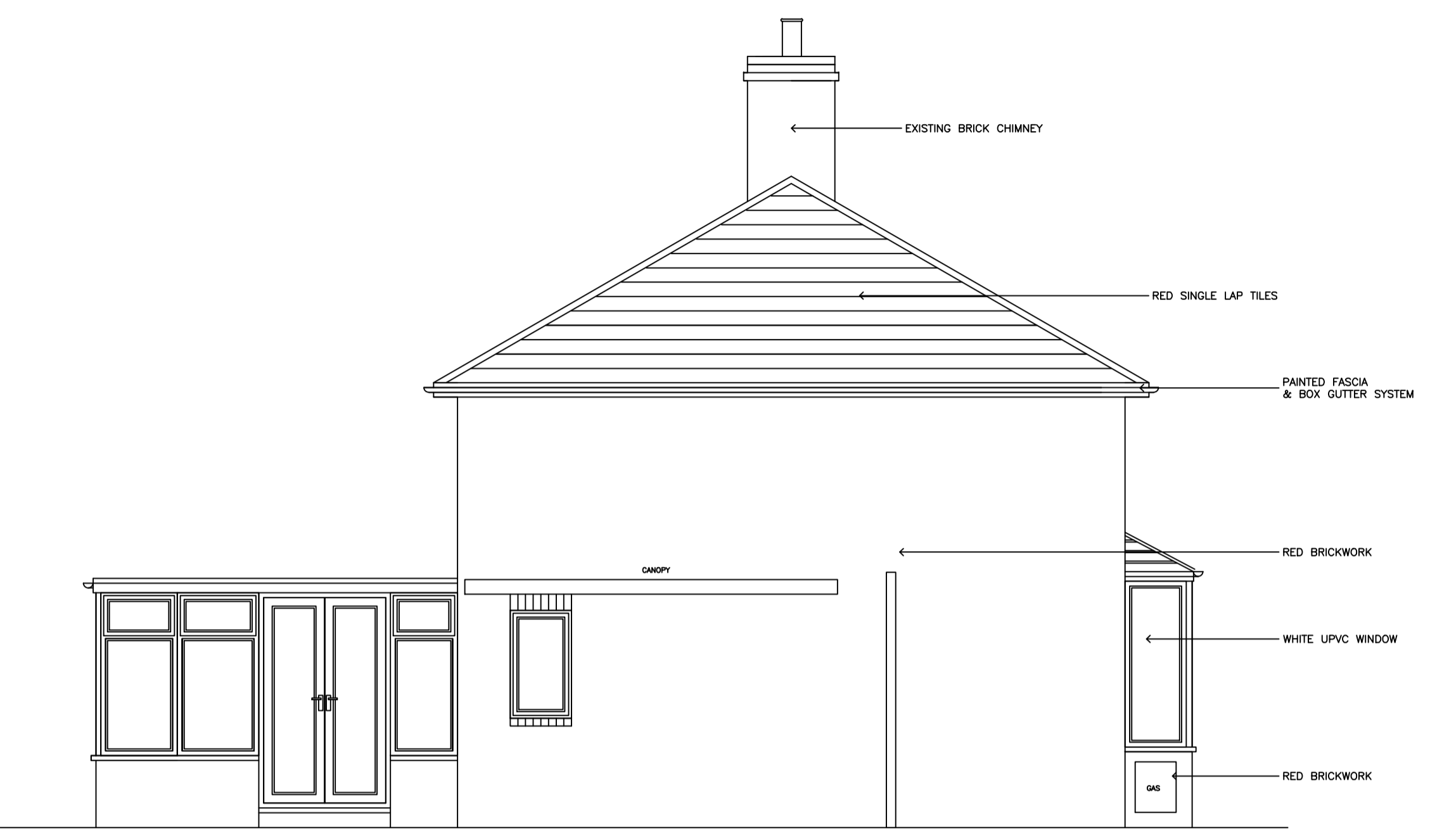
EXISTING EAST FACING ELEVATION (SCALE 1:50)
