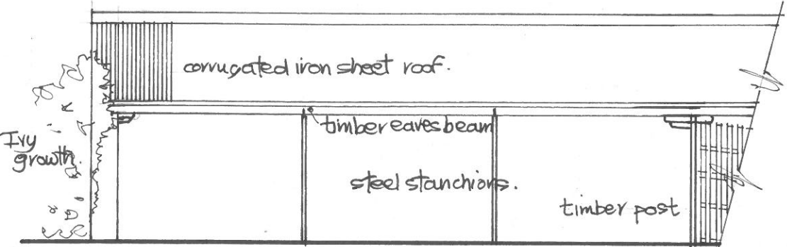
NORTH ELEVATION - EAST END CARTSHED 1:100.
