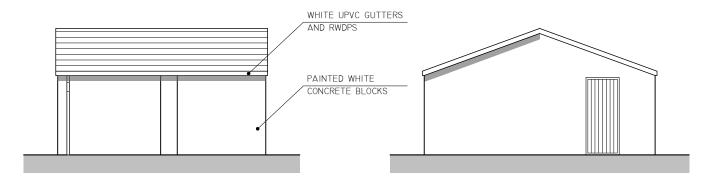
EXISTING SOUTH ELEVATION SCALE 1:100
