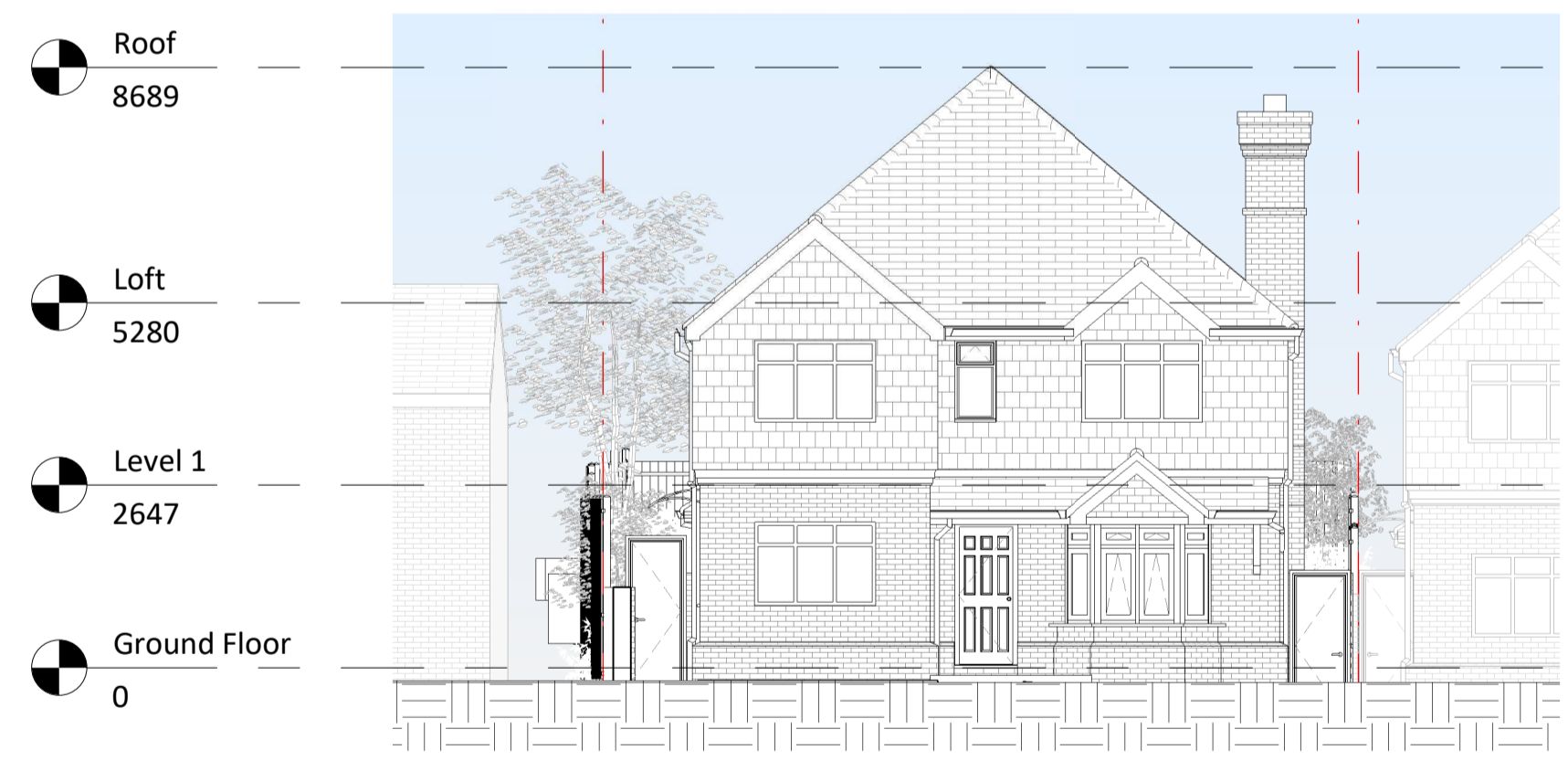
4 Existing Front Elevation 1 : 100
