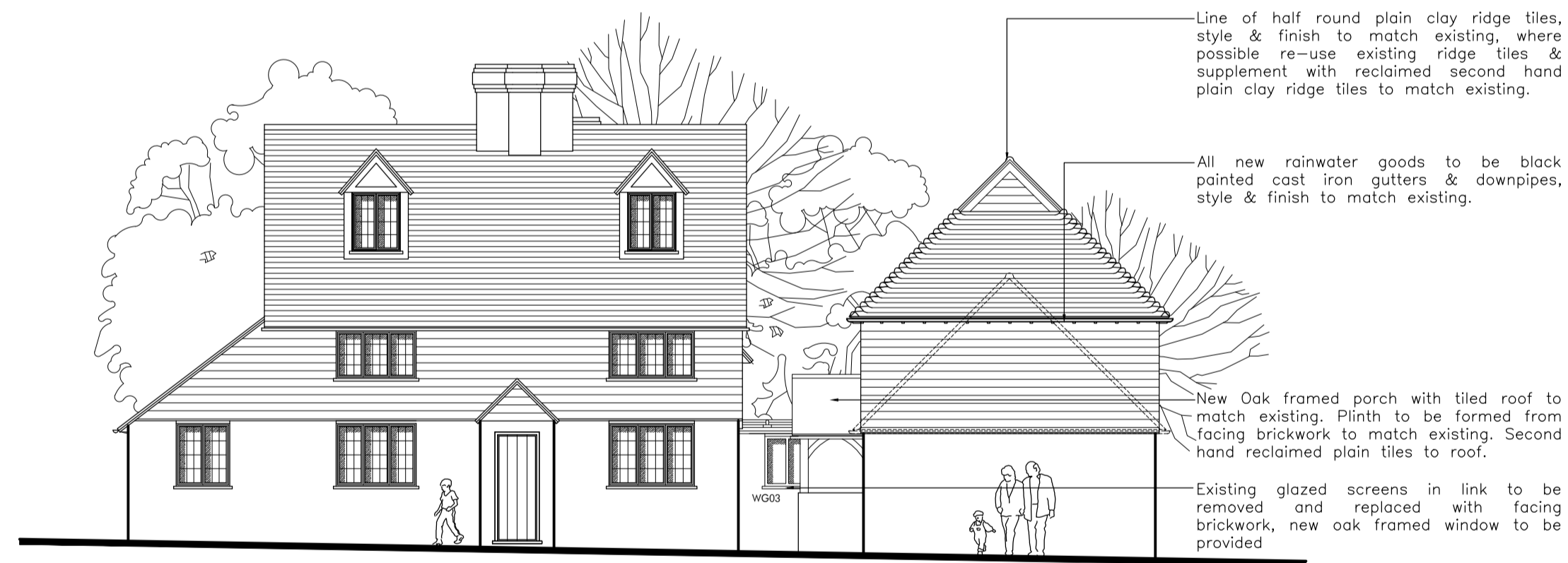
North West Elevation
