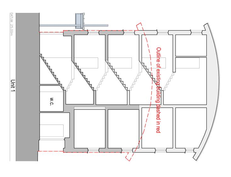
**Proposed section AA** Scale 1:100@A3 Refer to drawings 14 -18 for section references
