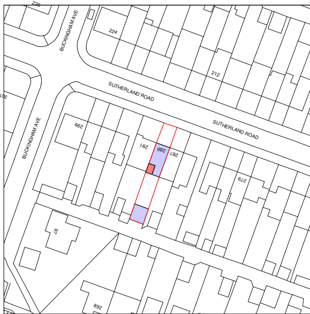
Existing Site Location Plan - Scale 1:1250 Existing denoted in Blue - Proposed denoted in Red.
