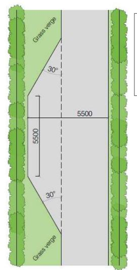
**Typical passing bay construction** Construct passing bay with a minimum overall depth of 450mm comprising of a minimum of 250mm sub base material, 100mm of bituminous macadam base course material, 60mm bituminous macadam binder course and 40mm bituminous wearing course
