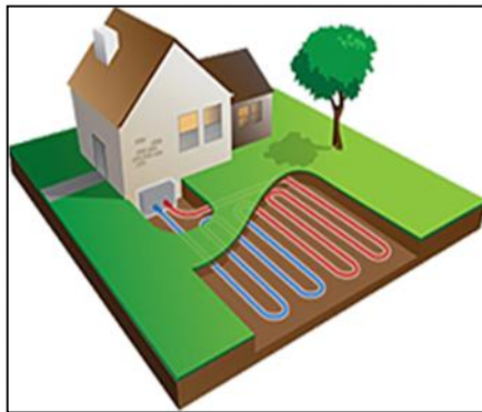
Horizontal Loop System
