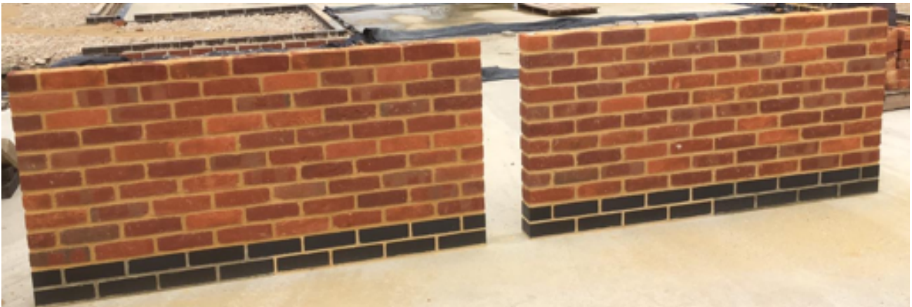
Image 1. Image of sample panels of proposed Swanage handmade bricks (red bricks only)
