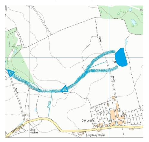
An uncontrolled release of water could only release 3,200 m3 of water, this would run into the existing field drainage system
