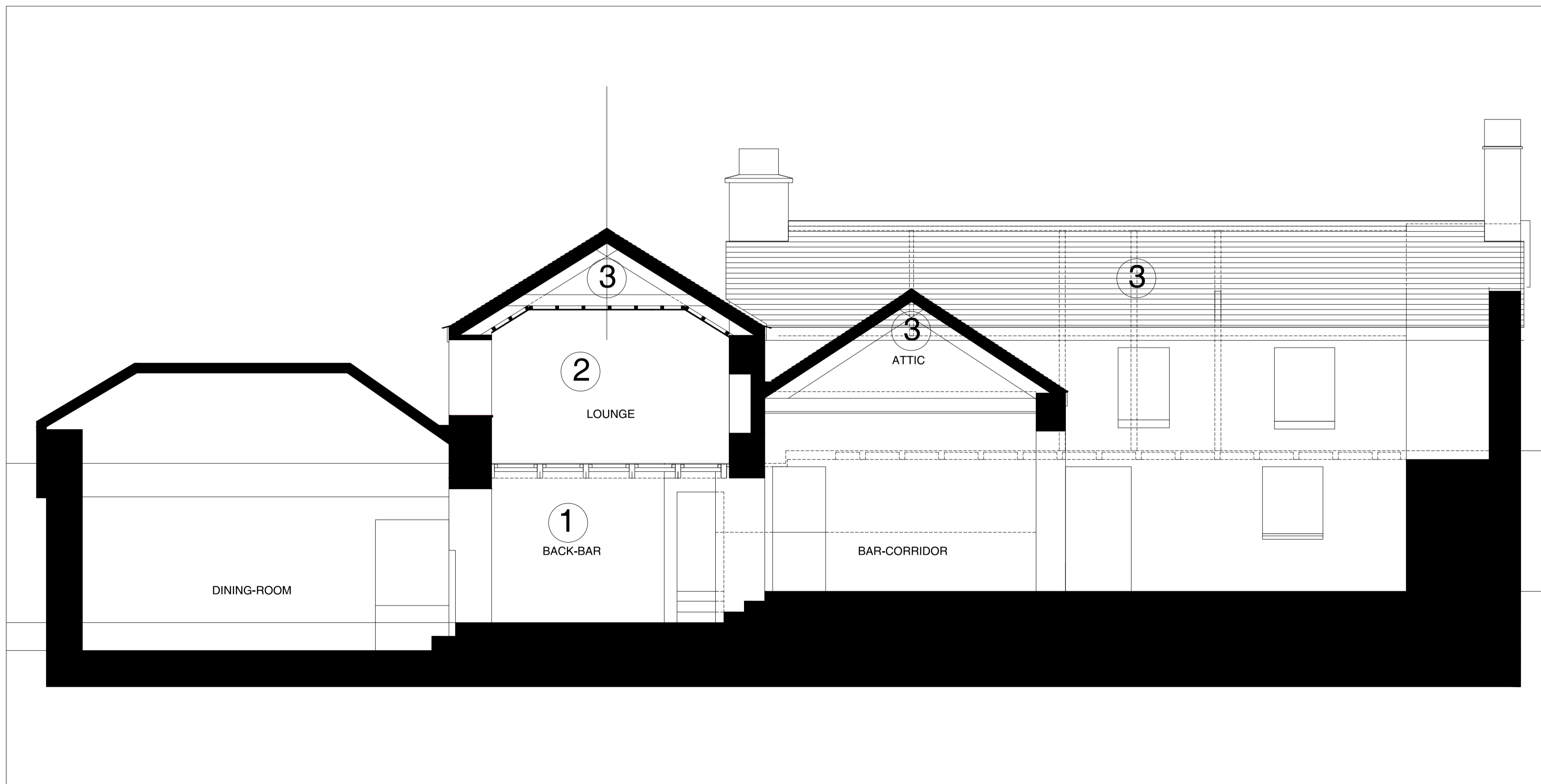
SECTION 2-2: THROUGH GROUND FLOOR BAR CORRIDOR 1:50@A1
