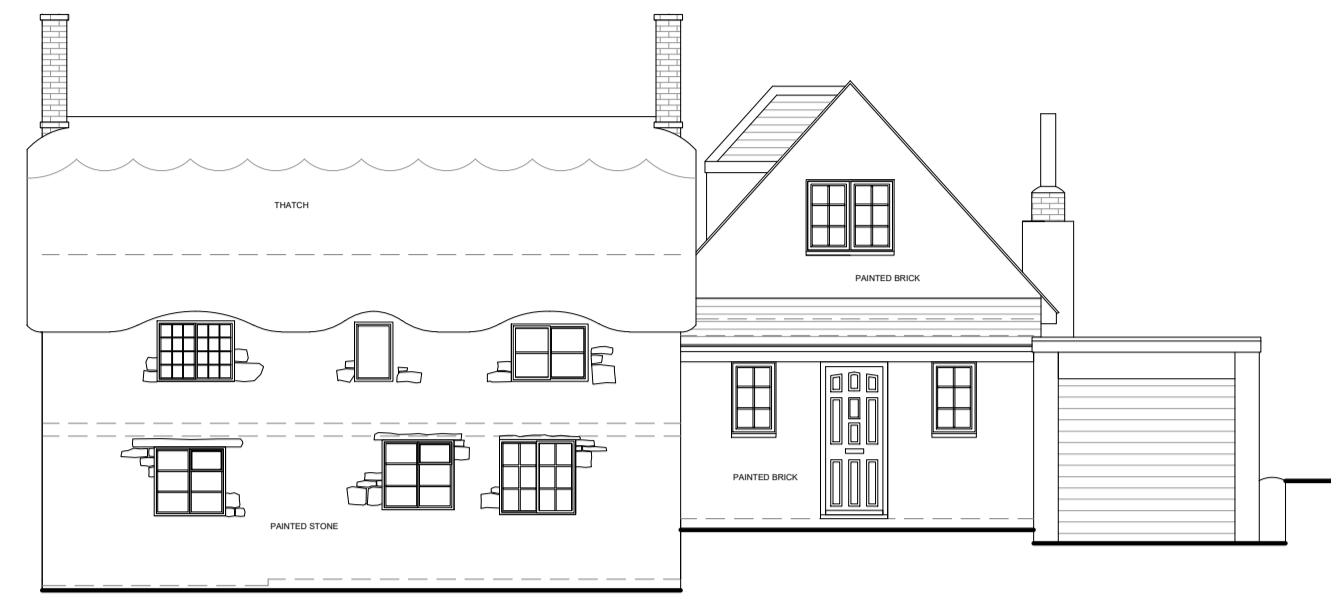
SOUTH EAST ELEVATION (Front)
