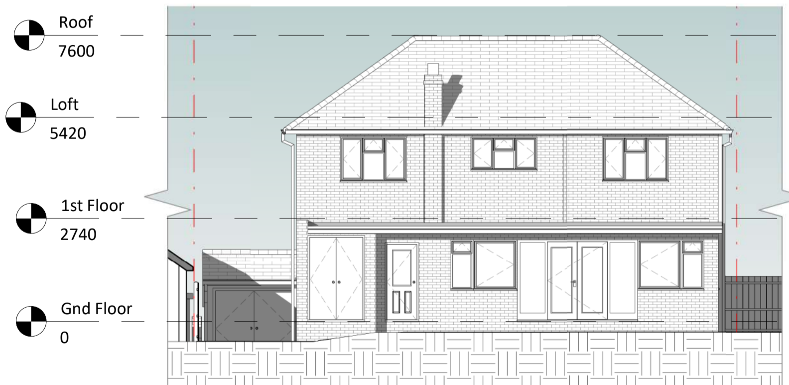
3 Existing Rear Elevation 1 : 100
