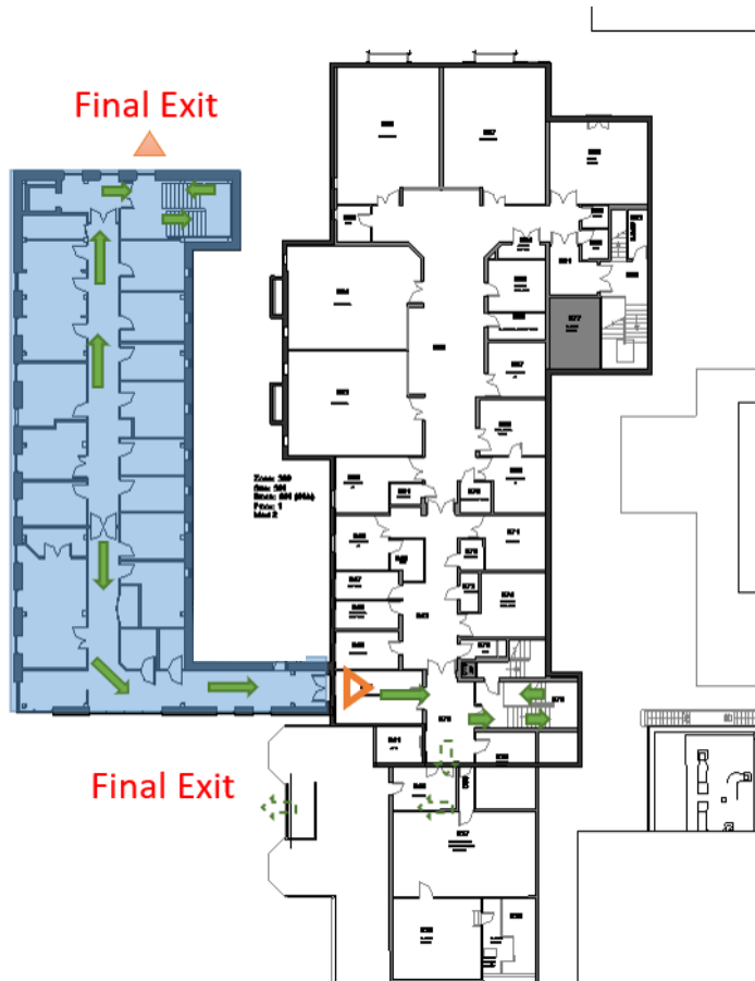
Figure 12: Means of escape from first floor
