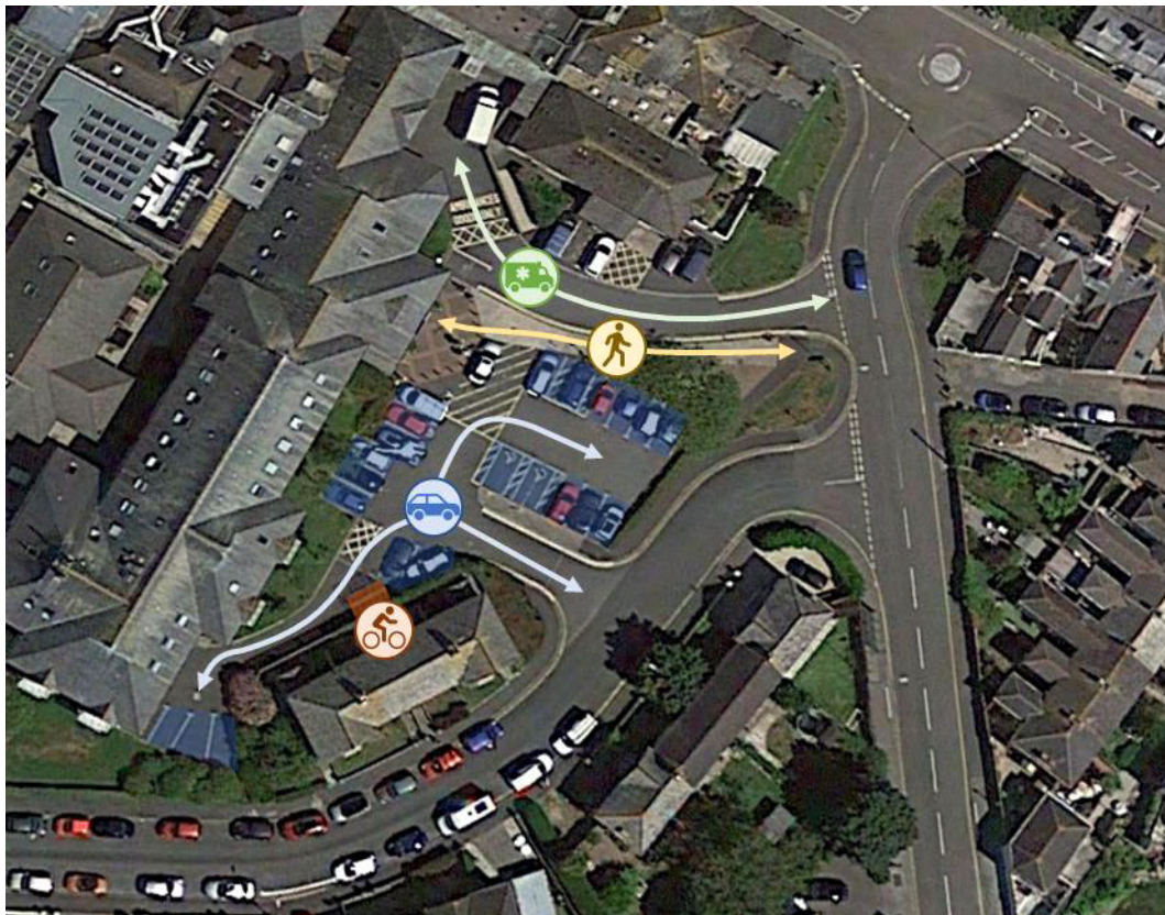
Figure 4: Access and Car Parking Existing Arrangement
