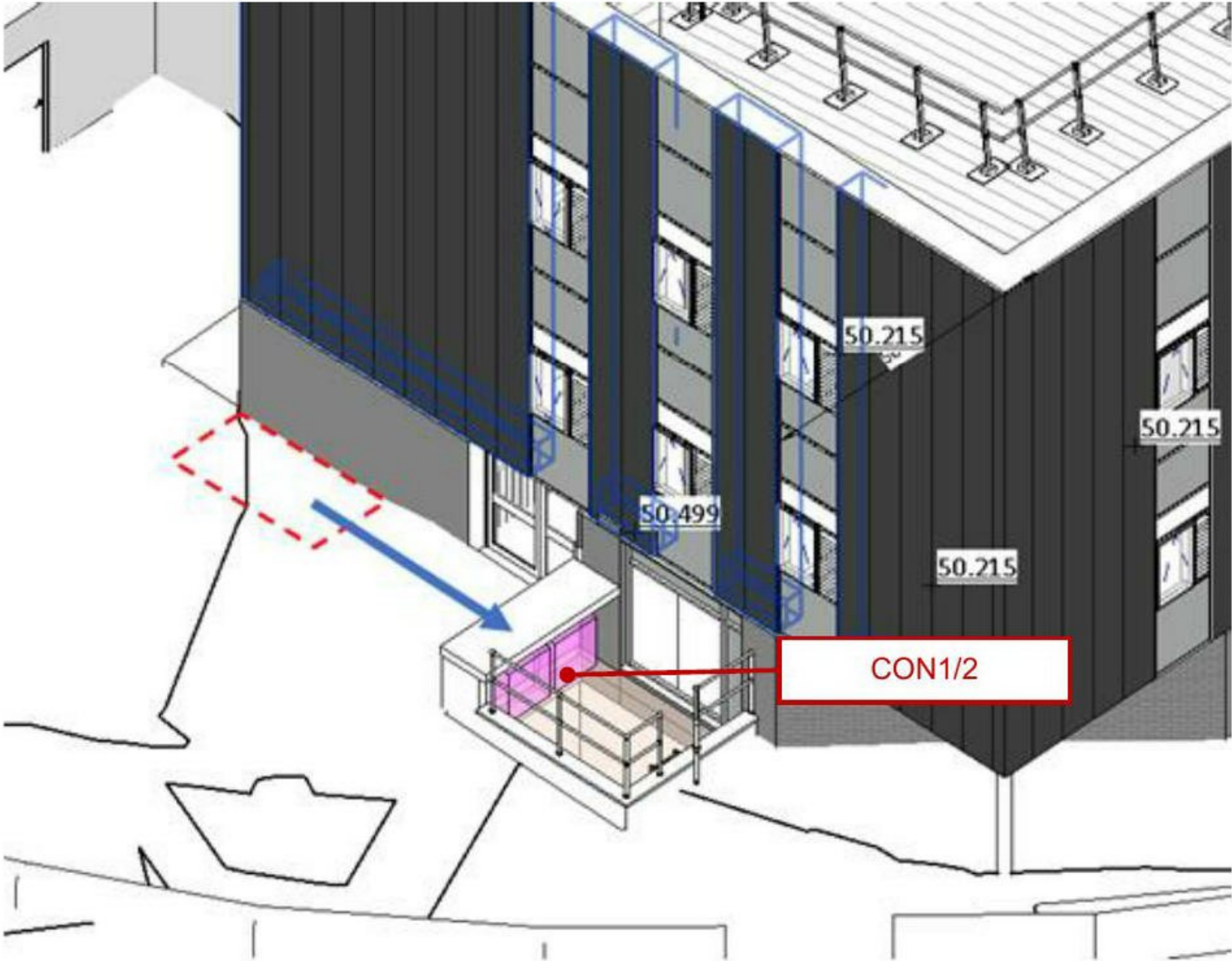
FIGURE 5: MODEL IMAGE INDICATING CONDENSER LOCATIONS (NOT TO SCALE)
