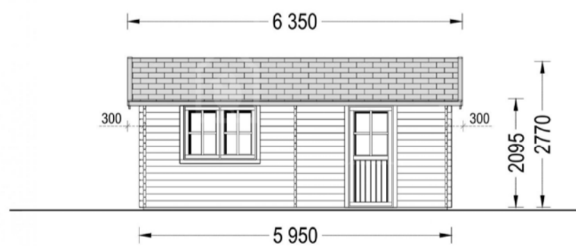
FRONT ELEVATION (Looking East)
