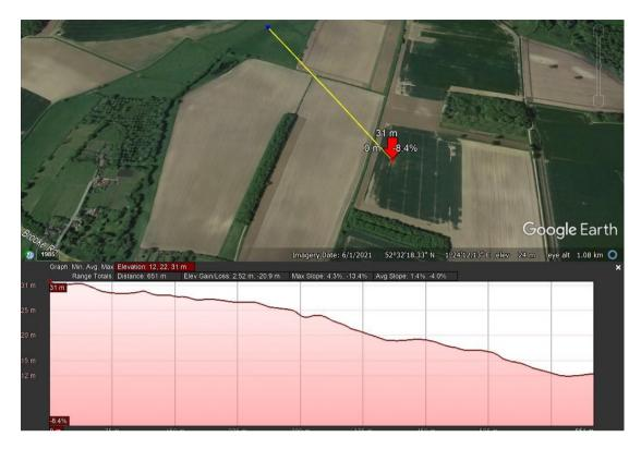
Flood way from theoretical breach in the NW corner, point of highest banks and slope to north west identified by topographical survey- see drawings.
