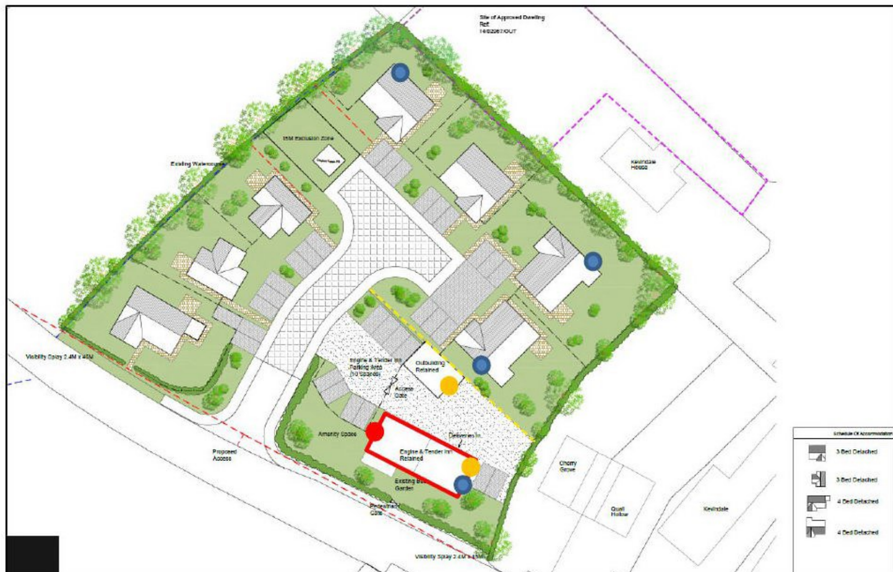
Figure 7. Locations of bat roosting features during and post works (during construction boxes - orange circles, post works bat tubes and large roost box – blue circles, recreated wall top roosting – red circle; and extent of roof void available for roosting bats – red rectangle)
