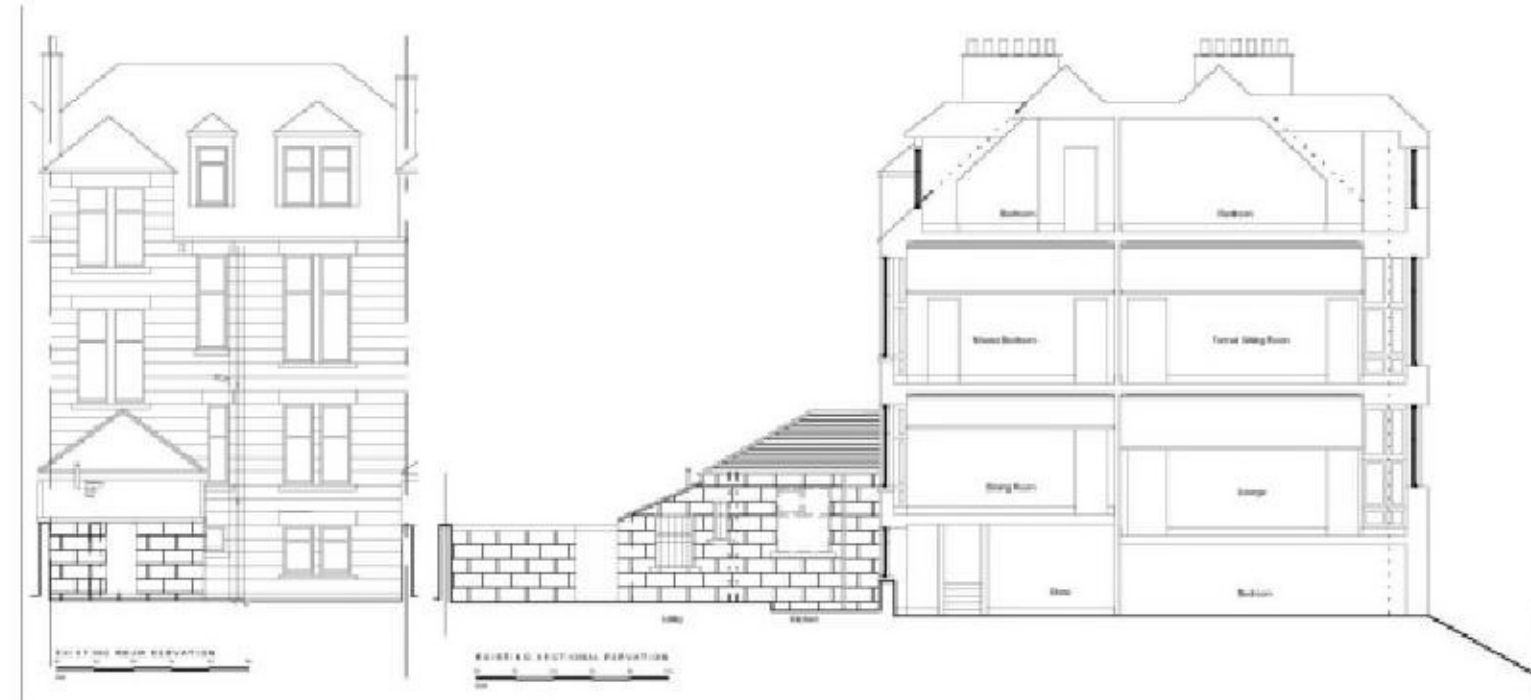
Existing Section and Rear Elevation
