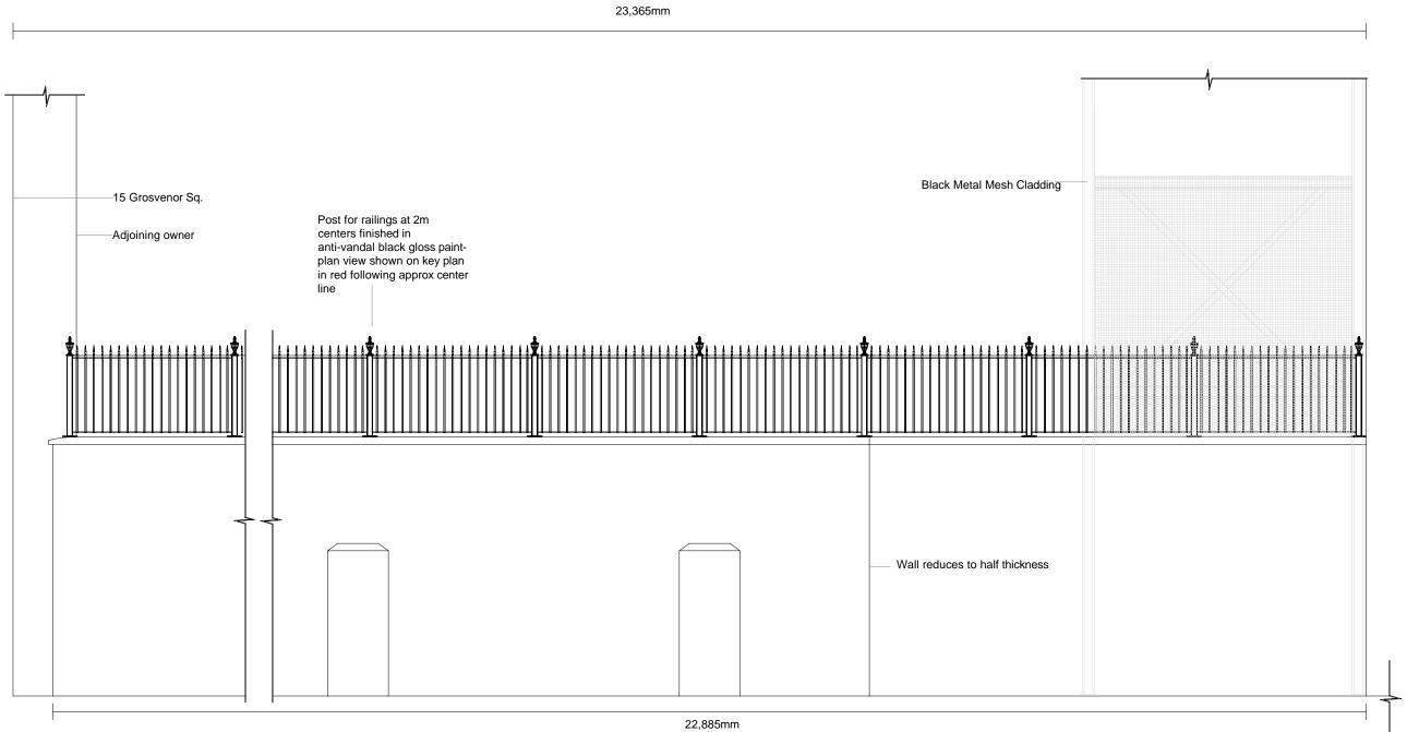
Proposed Boundary Wall Railings Section B-B
