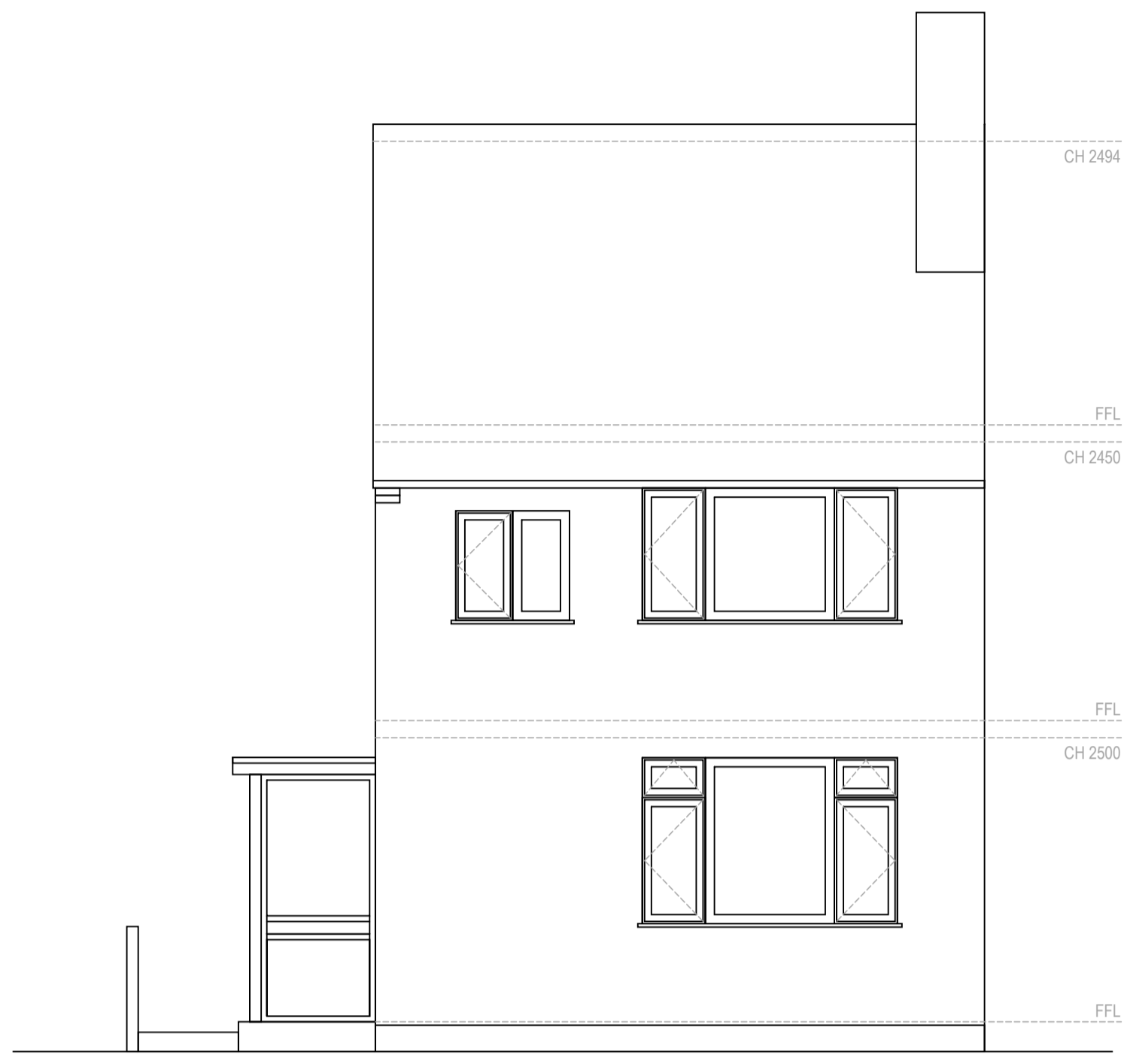
1 Existing Front Elevation 1:50 @ A1
