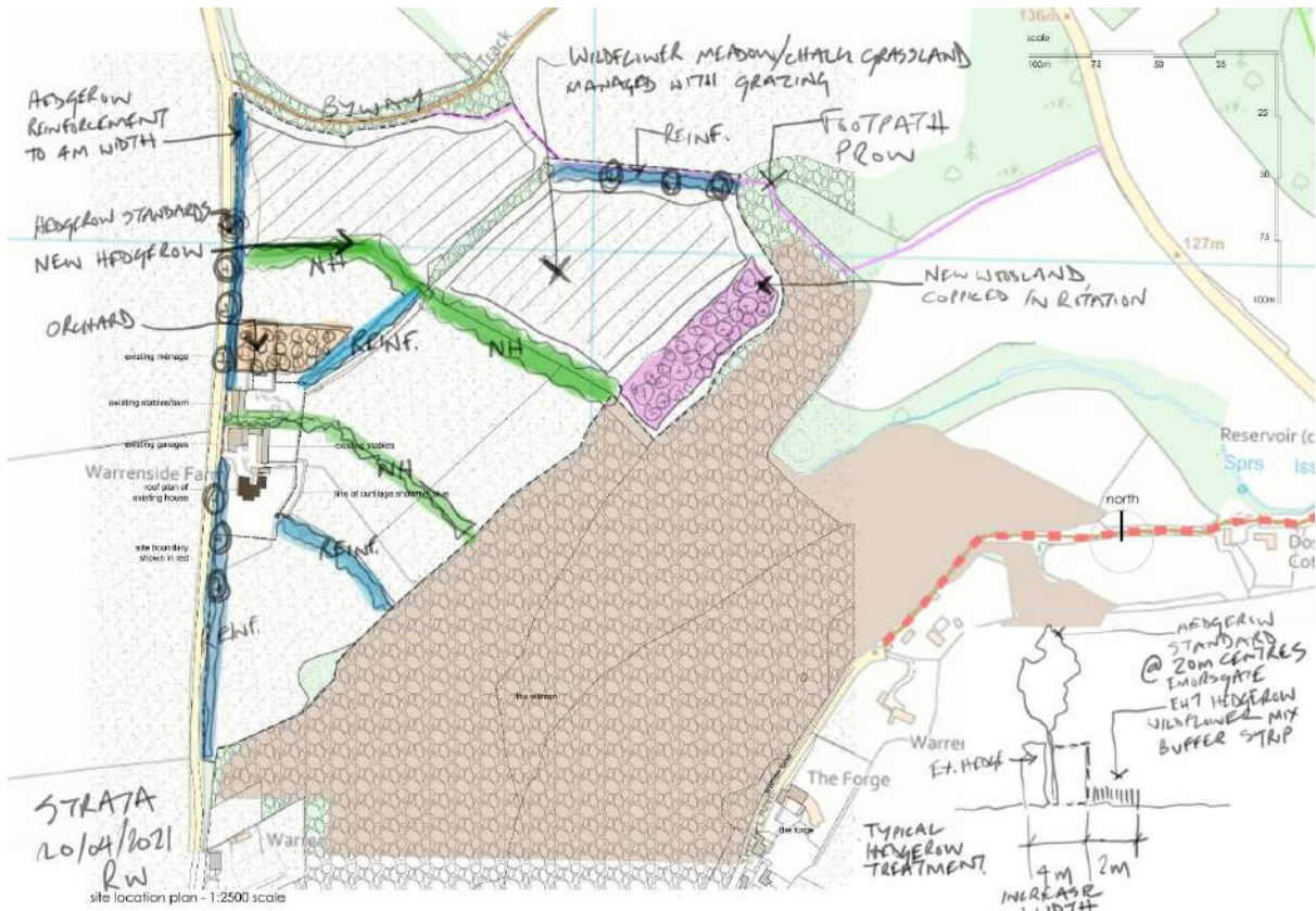
↑ Figure Seven – Outline of ecological enhancement measures to form part of the proposed development
