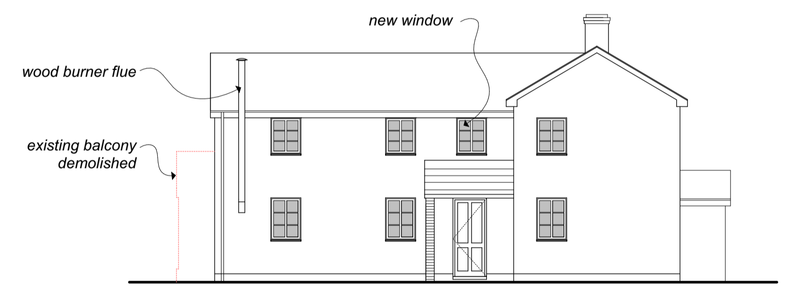
SIDE (NORTH) ELEVATION @ 1:100
