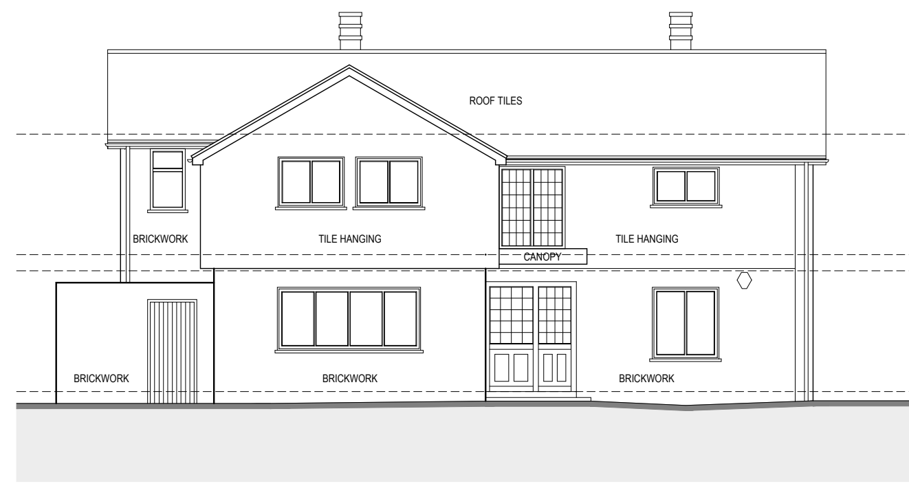
NORTH-WEST ELEVATION SCALE 1:100
