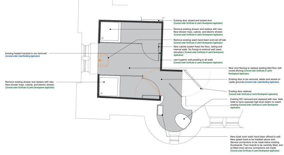
PROPOSED BATHROOM ALTERATIONS BATHROOM NUMBER : F04 & F05 (FIRST FLOOR, WEST WING)
